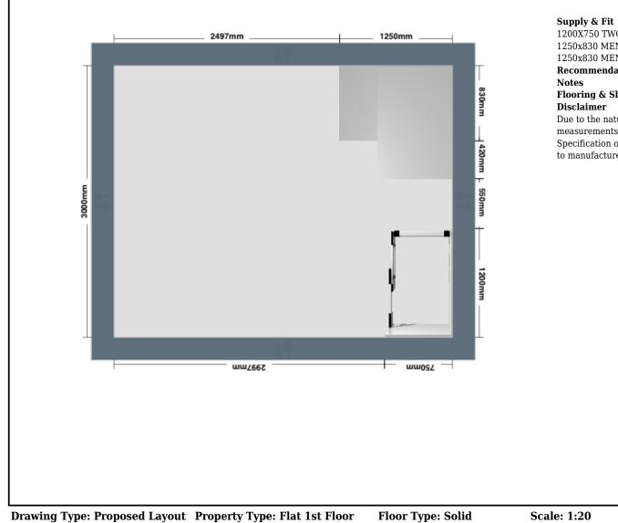
1200X750 TWO SIDED CUBICLE WITH OPTION H DOORS (RH) 1250x830 MENDIP THREE SIDED CUBICLE WITH OPTION G DOORS 1250x830 MENDIP THREE SIDED CUBICLE WITH OPTION G DOORS Recommendations
